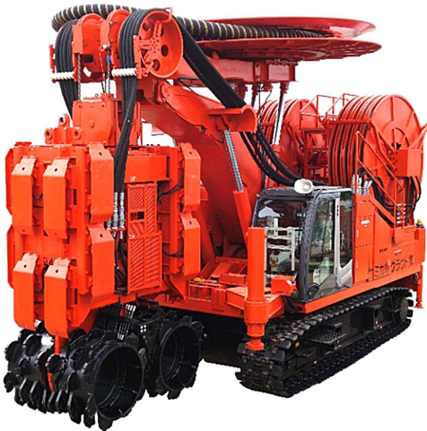
Diagonally parallel position for corner trenching
