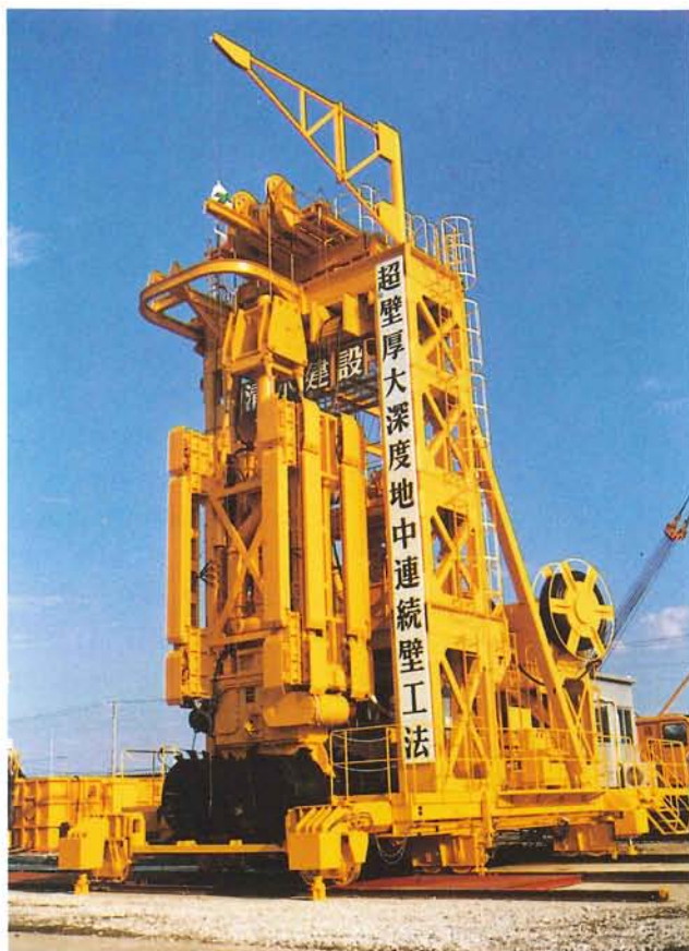
Derrick suspended Electro-Mill Drill (Shimizu Construction Co., Ltd.)
