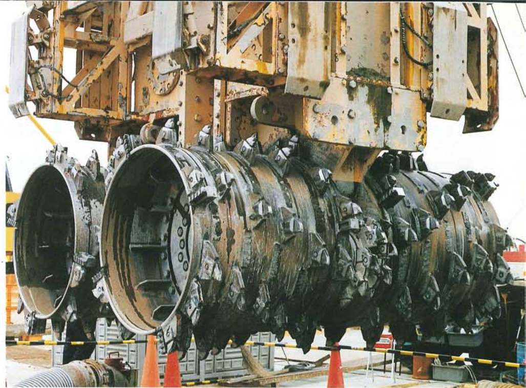
Drillhead consist of 4 drum cutters and 4 ring cutters.
